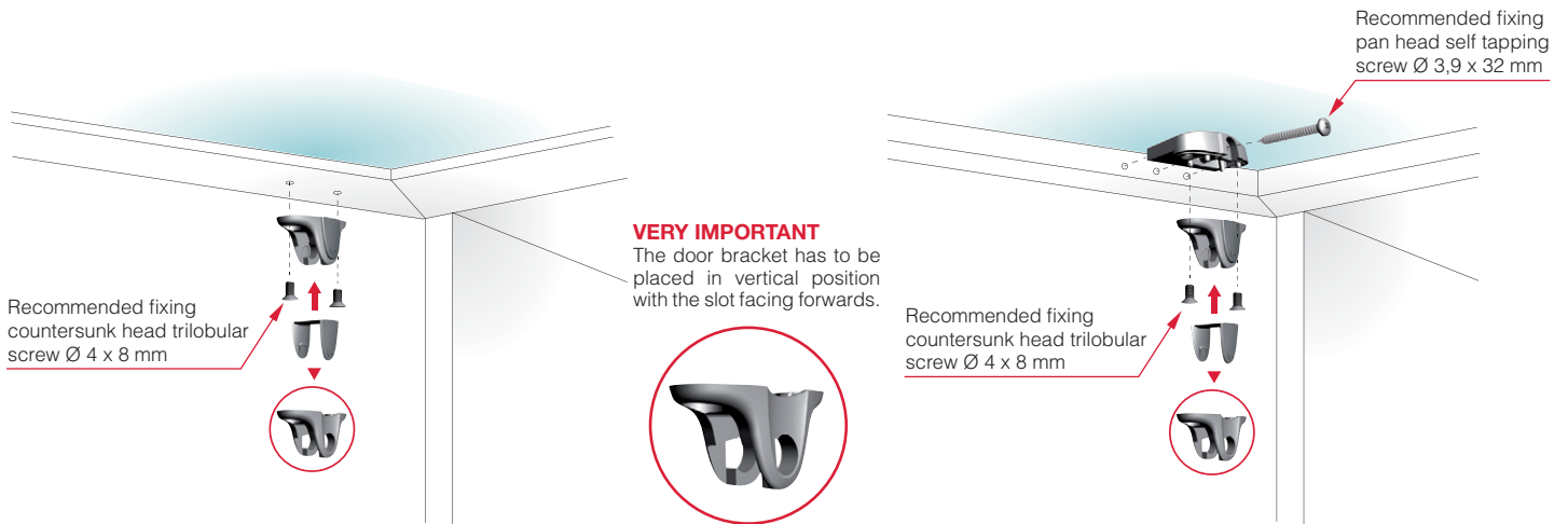
INSTALLATION ON WIDER ALUMINIUM FRAME DOOR
